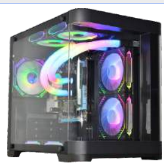
WATER COOLER INSTALADO
