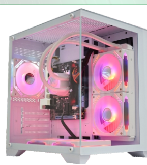
WATER COOLER INSTALADO
