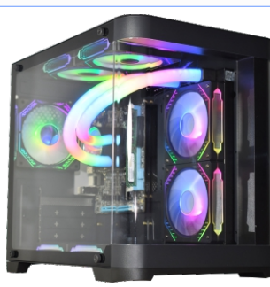
WATER COOLER INSTALADO
