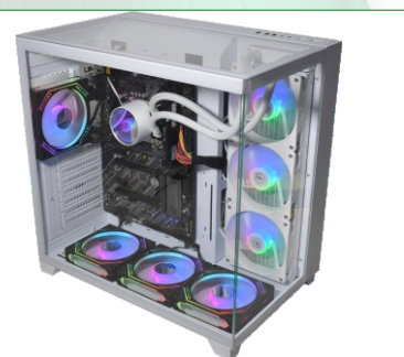
WATER COOLER INSTALADO
