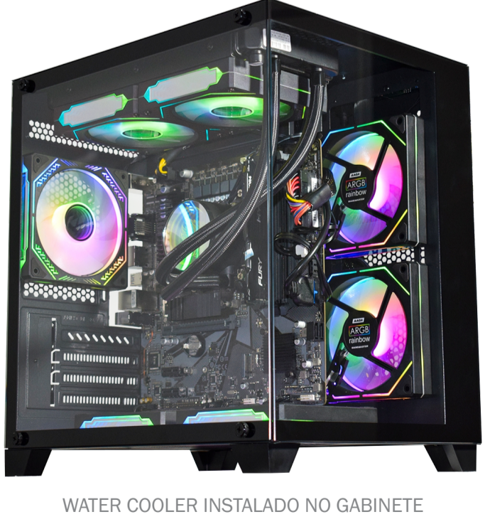
WATER COOLER INSTALADO NO GABINETE
