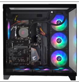
WATER COOLER INSTALADO
