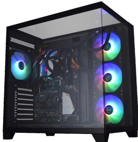
WATER COOLER INSTALADO NO GABINETE
