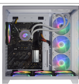
WATER COOLER INSTALADO
