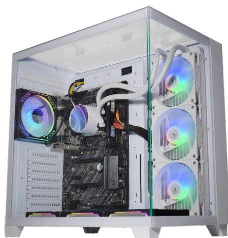
WATER COOLER INSTALADO NO GABINETE
