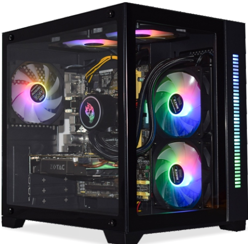
WATER COOLER INSTALADO NO GABINETE
